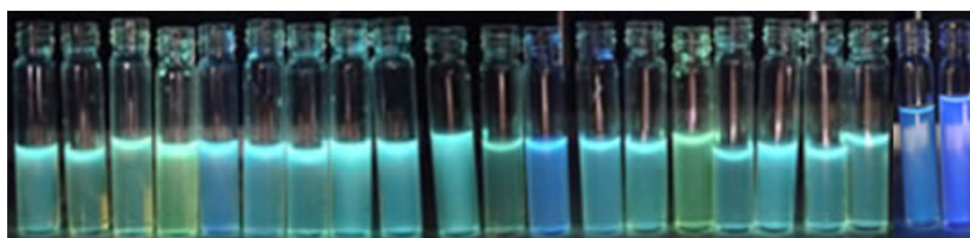
Figure. 2 The fluorescence of compound 6 under 360 nm ( 6a to 6u , left to right).
